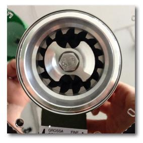
When adjusting the grind, what you are doing is moving the blades closer or farther from each other.
